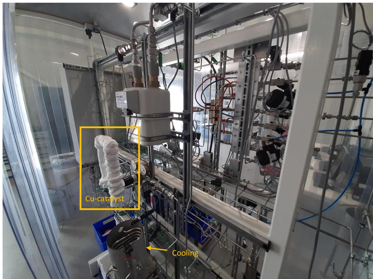
Figure 10 Set up of for the testing of the Cu catalyst
